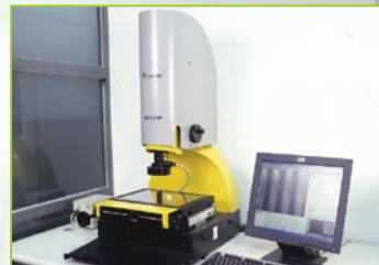
Video measuring microscope
