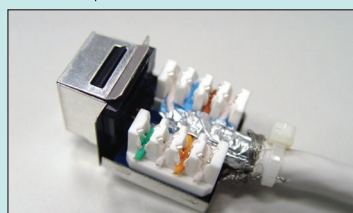
5. After termination completed, make sure the aluminum foil fully covers the wires all the way down to the block.
