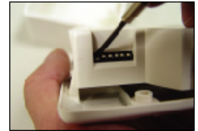
9. Select appropriate link mode from dip switch. Factory setup #1-5 is all on.
