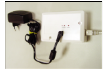
12. Use power adapter 5Vdc to power on, and connect the patch cord with RJ45 modular port.
